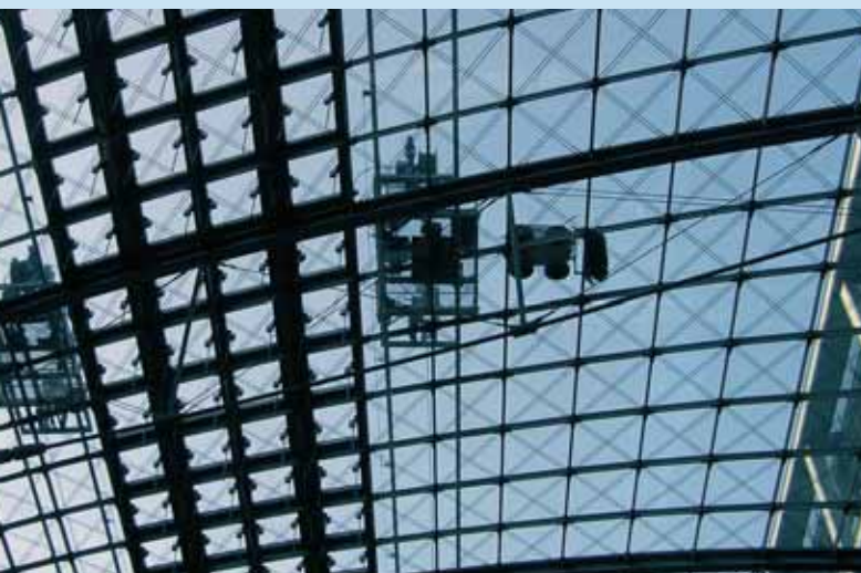
Service robot for the automated cleaning of glass roofs. Here, on the roof of Berlin Central Train Station.
