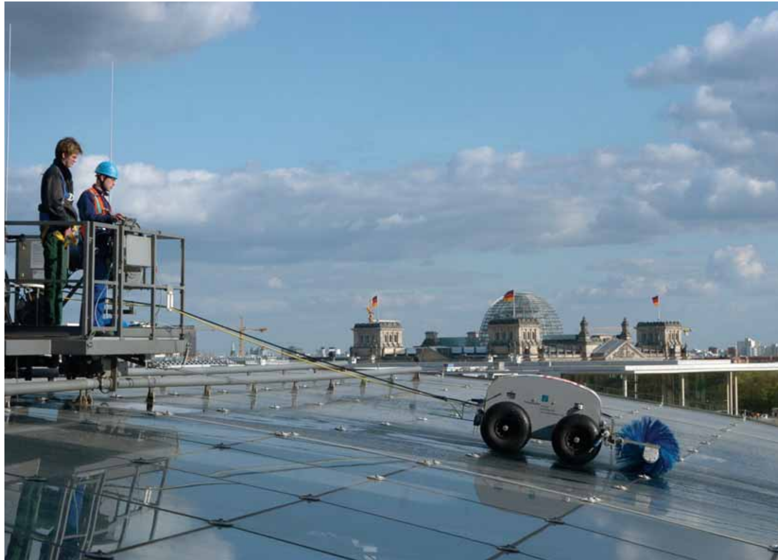
The cleaning unit Filius Toni keeps the view clear atop the roof of Berlin Central Train Station.
