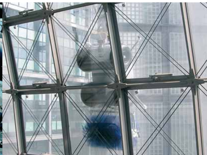
The cleaning unit Filius Toni in the eaves.
