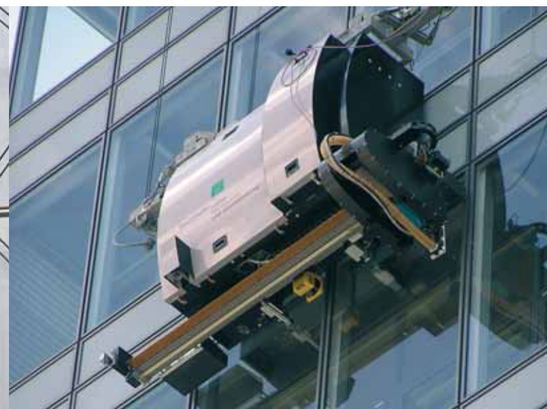
The fully automated cleaning robot SIRIUS ZV .
