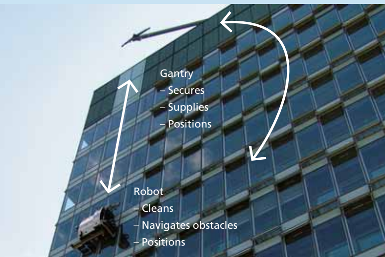
Basic modules of automated facade cleaning.
